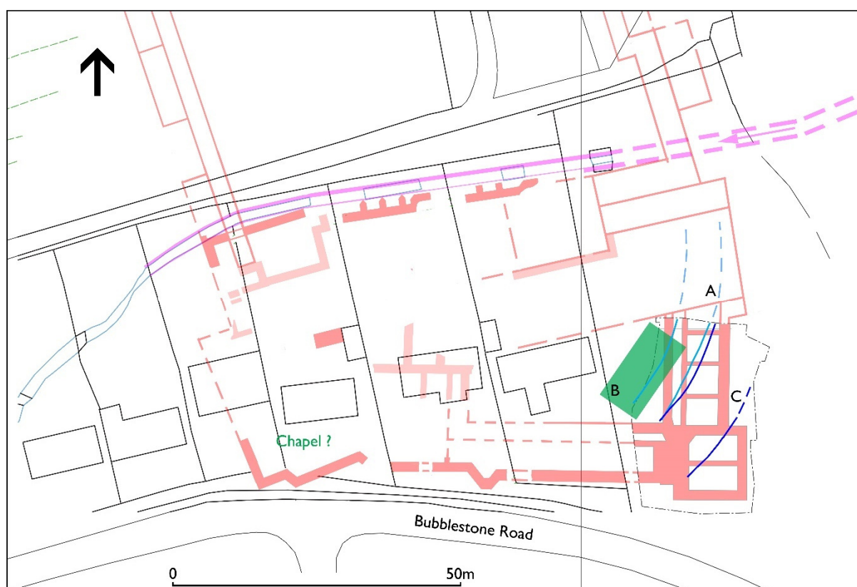
Fig 2 Elements of the earlier medieval house, in relation to modern development and (in red tone) known elements of the early 16th century palace. A, earliest moat; B, mid-14th century lodging range; and C, its associated moat, superseded by Warham's new south-eastern extension to the moated island
